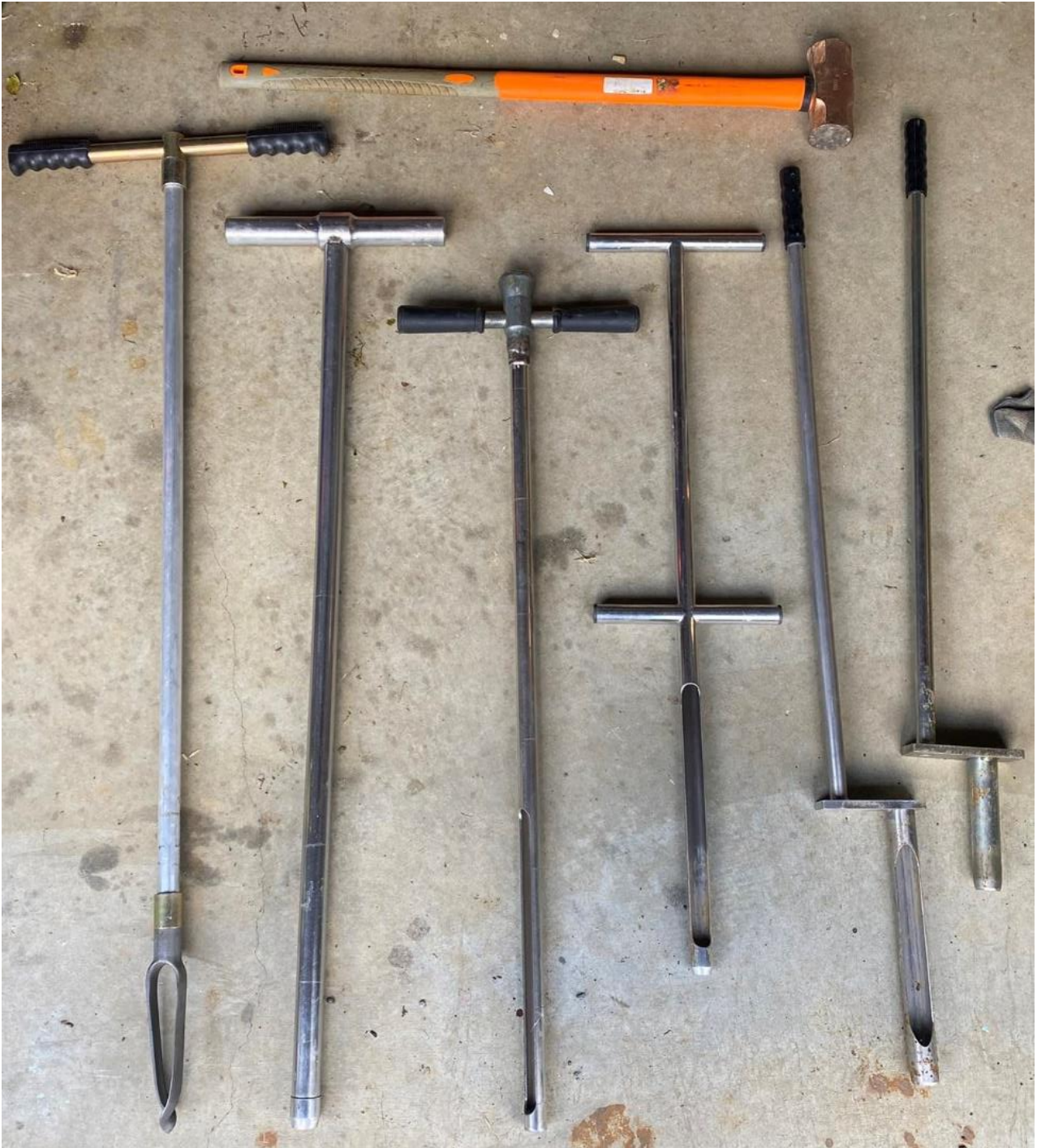
Figure 42. Examples of auger and corer types used during programme. From left to right: Dutch-head auger, PFR closed tube corer, Open-sided corer (hammer-type), Open-sided corer (push-type), 30 cm step-probe, 15 cm step-probe.
