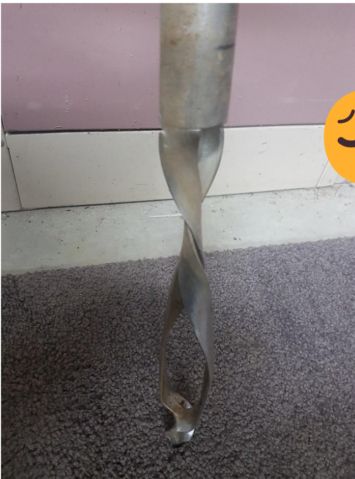
Figure 43. Examples of damaged and destroyed sampling equipment.
