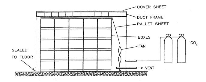
Figure 1. Typical CA tent layout for high CO<sub>2</sub> disinfestation of Asparagus.
