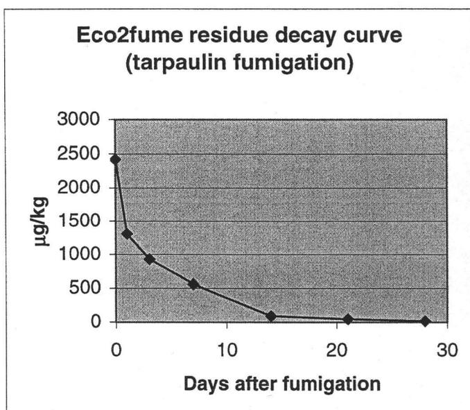
Figure 1: Phosphine residue decay curve for a fumigation carried out under a tarpaulin.
