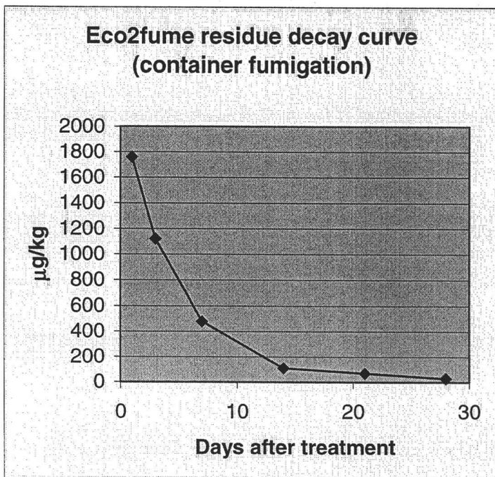
Figure 2: Phosphine residue decay curve for a fumigation carried out in a shipping container.
